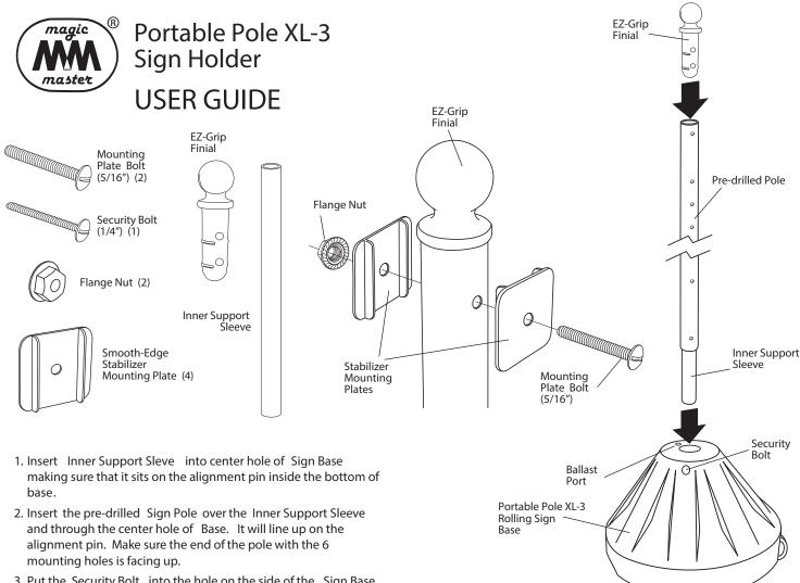
3. Put the Security Bolt into the hole on the side of the Sign Base and then rotate the Pole so that the holes line up with the Bolt. Screw in firmly making sure that it fits in the hole in the Pole. The Pole may need to be turned or lifted slightly to ensure that the Security Bolt is properly seated. Do not overtighten.
